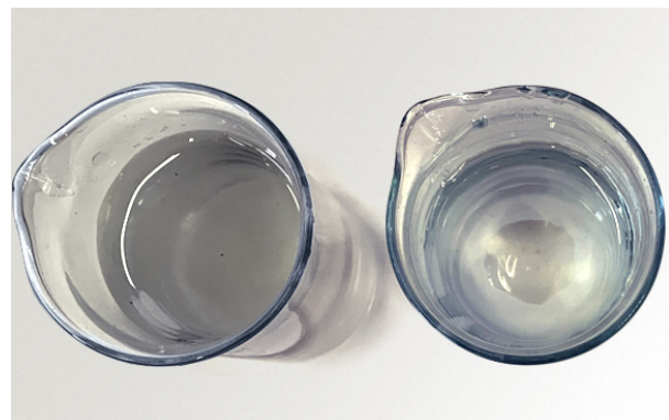
Left: Feed sample before filtration; right: filtrate sample after filtration. © FiW e. V.
